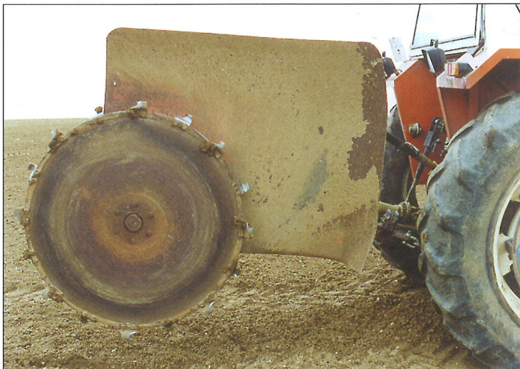
Photo 3 - Drain machine of artisanal manufacture.
