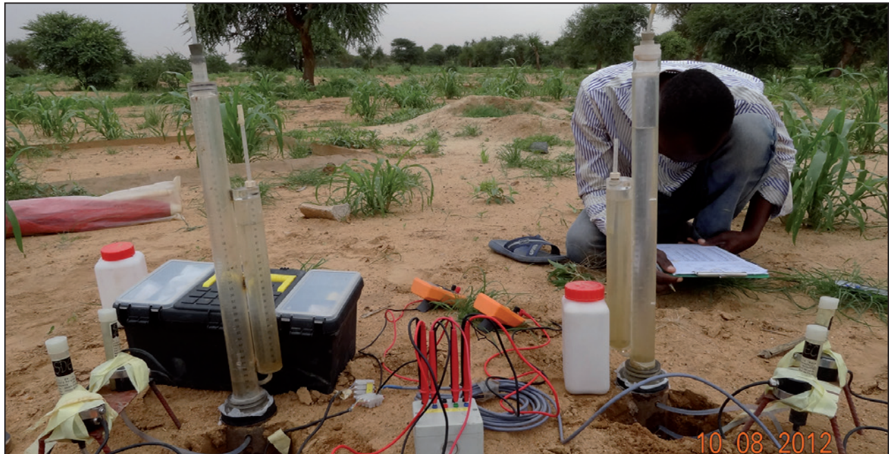
Figure 4 - Infiltration measurement progress on a field, close to runoff plot (behind). Each infiltrimeter, located upon a previously installed cylinder, is monitored by an observer who reads regularly (each minute at least at the beginning) the water level in the reservoir, as well as signal emitted by tensiometers, read on digital voltmeters.
